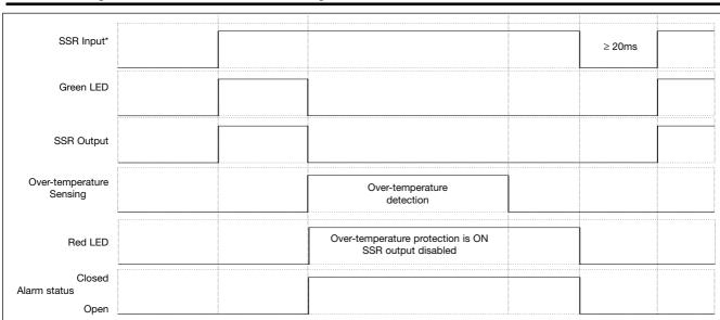
\*After over-temperature condition is removed, SSR can be reset by switching OFF the control input for more than 20 ms and switching back ON: this will switch ON the SSR output
